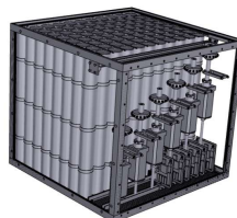
Schematic view of the 88 sample cylinders inside the HIRES (High Resolution Sampler)
